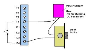
B. **DC Silent:** Connect the strike across D1 and D2 terminals and use a Class 2 transformer; connecting to terminals T3 and T4 (as shown below). This method utilizes unit's internal rectifier to provide silent operation using an AC transformer.
