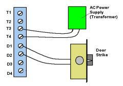
C. **AC Buzzing:** Connect the door strike across D3 and D4 and transformer across T3 and T4 (as shown below). Transformer output is not rectified.
