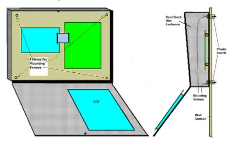
Carefully mark these holes on the wall, at an appropriate height from floor for easy access. Drill and install plastic inserts (if required). Then, using four self-tapping or wood screws, secure the unit to the wall.
