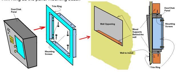
Carefully inspect the Trim Ring to plan the wall opening. The opening should be 19 5/8"x 13 5/8" and 2 1/4" deep so that the trim ring fits properly.
