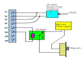
NOTE: Do not exceed maximum switched strike load of 28V @ 3 Amps in any of above connections.
